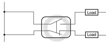
Connect the load to the same polarity.
