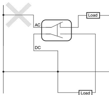
Do not design a circuit where voltage is imposed between contacts, otherwise contact weld may result.
