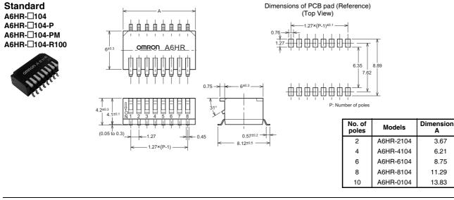
Note: Unless otherwise specified, a tolerance of ±0.4 mm applies to all dimensions.
