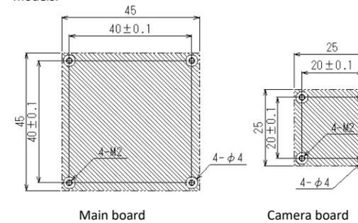
Do not install metallic parts for mounting on the shaded areas.
