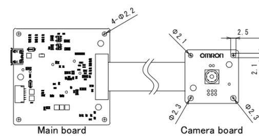
1. This figure is for a frontal mounting direction (0°) of the module. Settings need to be changed through commands when mounting the Device at a clockwise rotation angle of 90°, 180° or 270° from the front.
